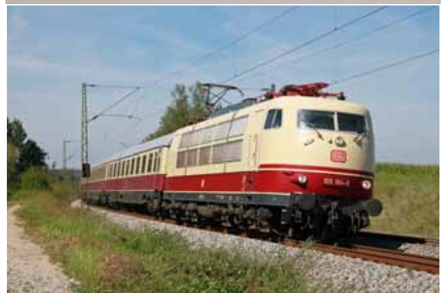
The DB E-103 Heavy Passenger Express, built between 1966 & 1973, delivered over 10,000hp. 149 were built and the last in regular service was in 2003.
