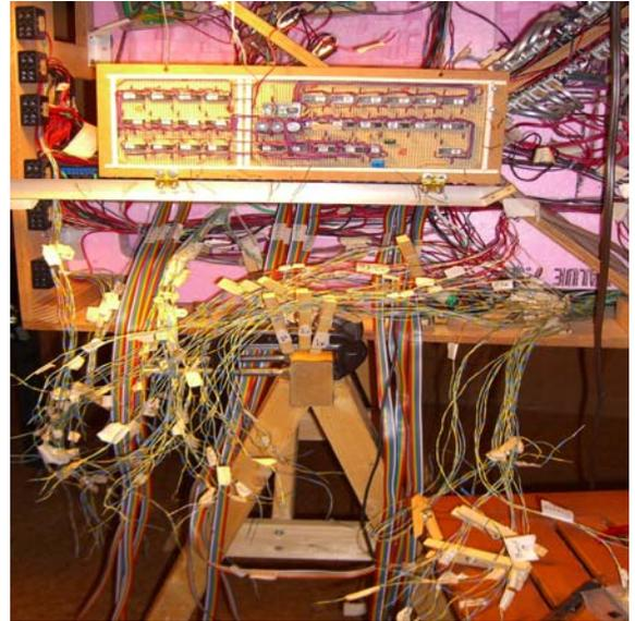
Photo above shows the PCB hung temporarily near the tangle of about 56 input wires and about 109 output wires ready to be trimmed and connected (soldered) to either the input or output shift registers. The module is on its back lying across two saw horses. The PCB is vertical so I can push wires through the holes in the board. The PCB is then rotated to a horizontal position to facilitate soldering the wires to the board.
