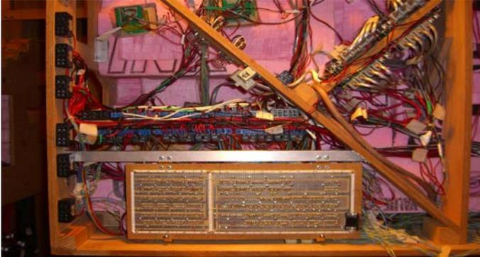
Above photo shows the PCB hinged and locked in place. All the wires and components are hidden. All you can see is the back side of the board with about 1,180 solder connections.
