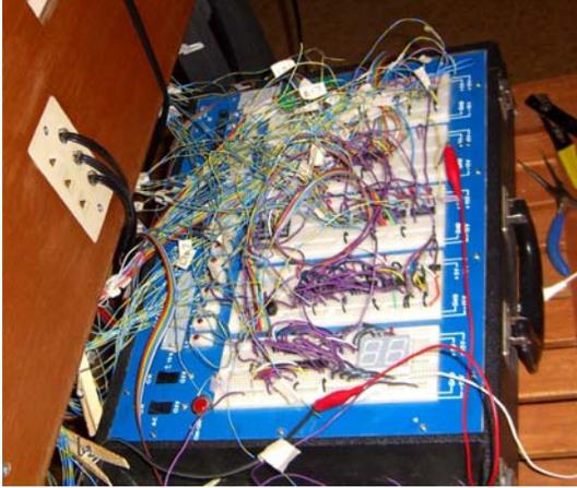
and software for the lower loop. I then made changes to the breadboard and tested the hardware and software for the middle and upper loops in a similar way. The next step was to populate and wire the PCB exactly the same as the breadboard tester so that the electronics would become an integral part of the portable module.
