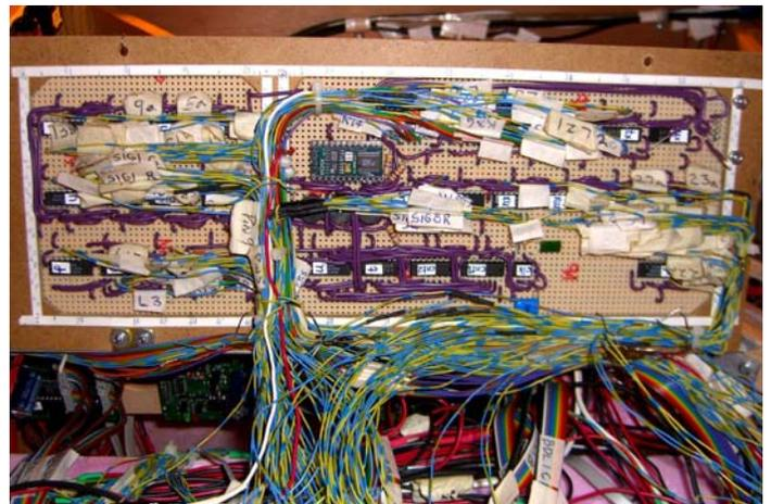
Photo above shows all the input and output wires connected to the PCB. The PCB is on its hinged
