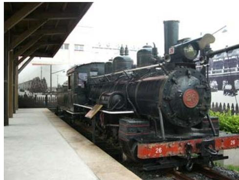
A SN-26, 0-5-0 type steam locomotive built in the USA in the 20's specially for running on narrow gauge railroads. It retired in the 1990s after around 60 years of service in the mountainous areas of Yunnan Province.
