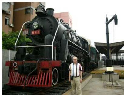
A SN-26, 2=4=0 type steam locomotive built in the USA in the 40's specially made for running on narrow gauge railroads. It retired in the 1990s after about 50 years of service in the mountainous areas of Yunnan Province.
