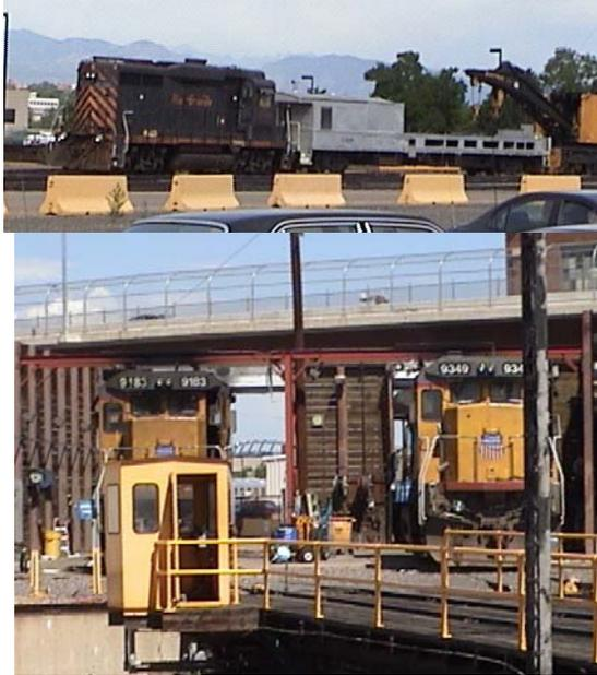
The shops can repair up to 10 locomotives per day. Outside the building there is a test area near the old turntable. This tester checks out locomotives under load and checks how much exhaust it is putting out. The locomotive then is returned to service.
